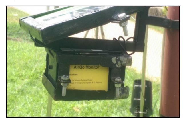
The AirQo monitor is designed to monitor PM 2.5, and PM 10, location details, internal and external temperature, atmospheric pressure, and humidity.
