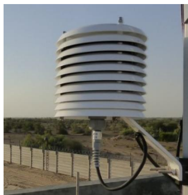
Figure 7: Temperature sensor in protective case
