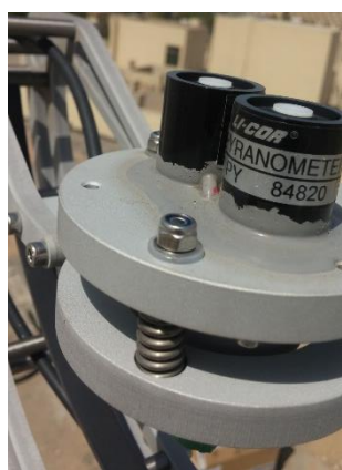
Figure 3: Pyranometer Unit on RSI
