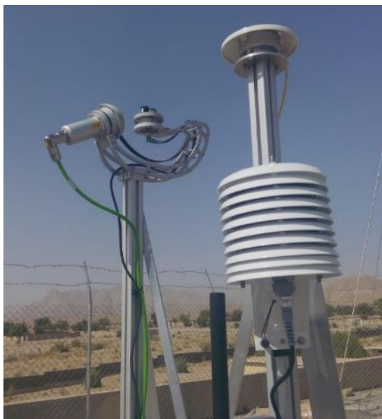
Figure 7: Temperature sensor in protective case (white), GPRS antenna (black), RSI and pyranometer
