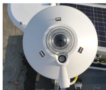
Figure 4: CMP10 w. sun shield
