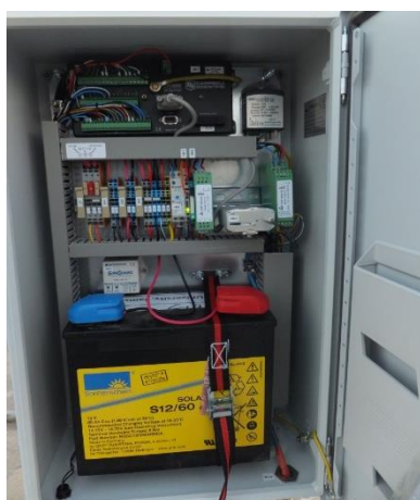
Figure 3: Control box with datalogger, battery and electric equipment
