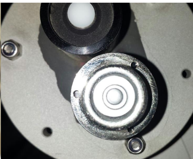
Figure 4: RSI horizontal leveling
