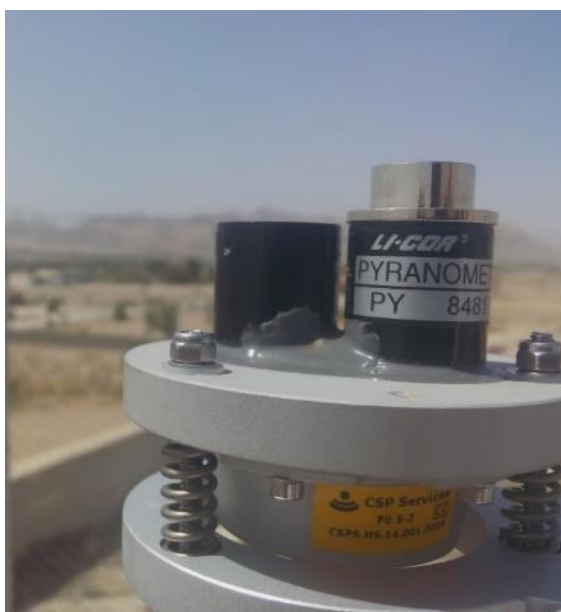
Figure 3: Pyranometer Unit on RSI (with water level on top)
