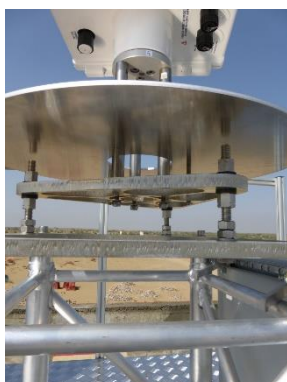
Figure 13: Tracker mounting
