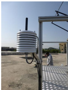
Figure 7: Temperature sensor in protective case (white), GPRS antenna (black)
