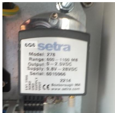
Figure 2: Setra 278 pressure sensor
