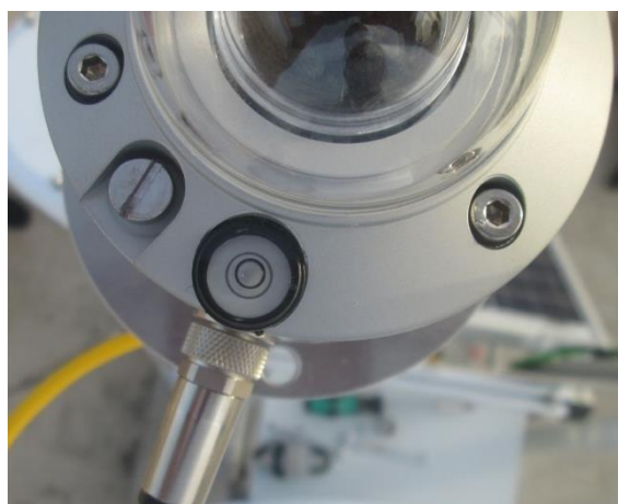
Figure 13: Pyranometer leveling
