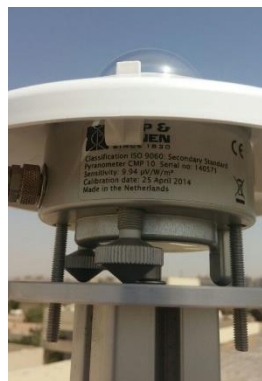
Figure 2: CMP10 w. sun shield
