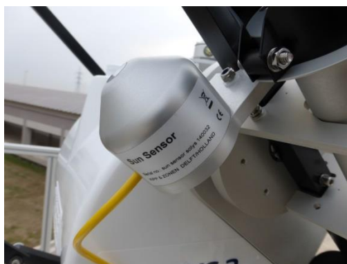
Figure 6: Sun sensor for active tracking control
