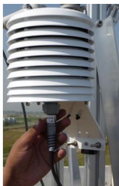
Figure 7: Temperature sensor in protective case
