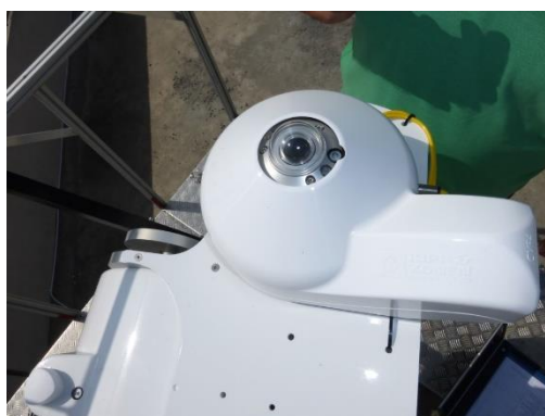
Figure 4: CMP21 w. CVF4 ventilation unit
