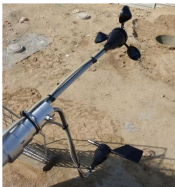
Figure 1: Wind Speed and Direction Sensor
