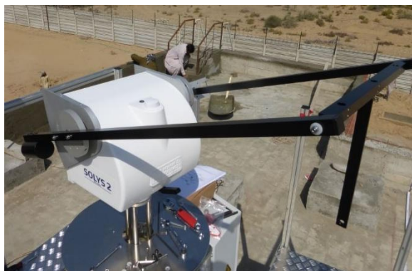
Figure 2: Solar tracker with shading ball assembly, without sensors
