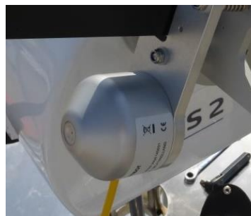
Figure 6: Sun sensor for active tracking control
