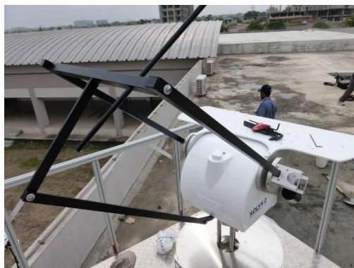
Figure 2: Solar tracker with shading ball assembly, without sensors
