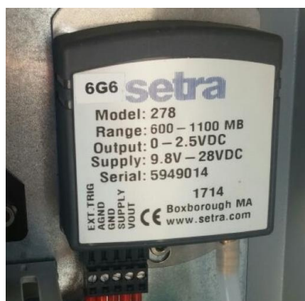
Figure 4: Setra 278 pressure sensor
