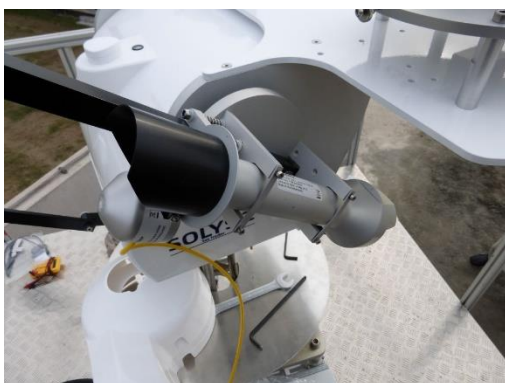
Figure 5: CHP1 on tracker
