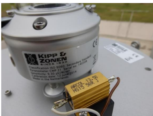
Figure 3: CMP21 close-up, w. heating element of vent. unit
