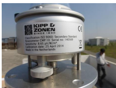
Figure 3: CMP10 close-up, w.o. sun shield
