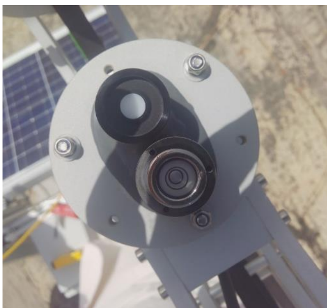
Figure 4: RSI horizontal leveling
