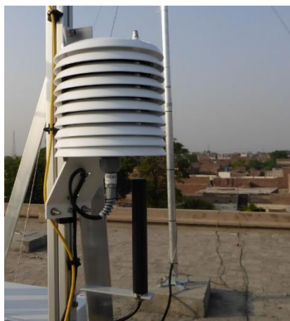
Figure 7: Temperature sensor in protective case (white) and GPRS antenna (black)
