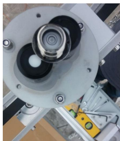
Figure 4: RSI horizontal leveling
