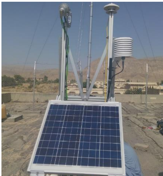
Figure 5: Support structure with PV panel and sensors
