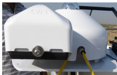
Figure 4: CMP21 w. CVF4 ventilation unit
