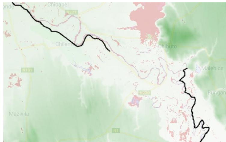
Figure 15 Channel dynamics for a section of Limpopo river. Red areas depict satellite detected wet areas. The Black lines show the locations of dikes.
