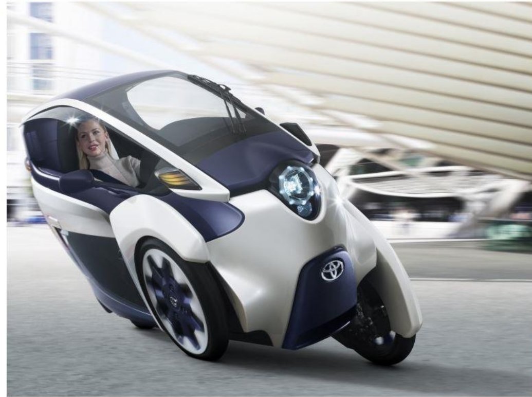
Toyota's i-ROAD is a fully-enclosed, two-seater, three-wheeled, fully-electric, Personal Mobility Vehicle (PMV)
