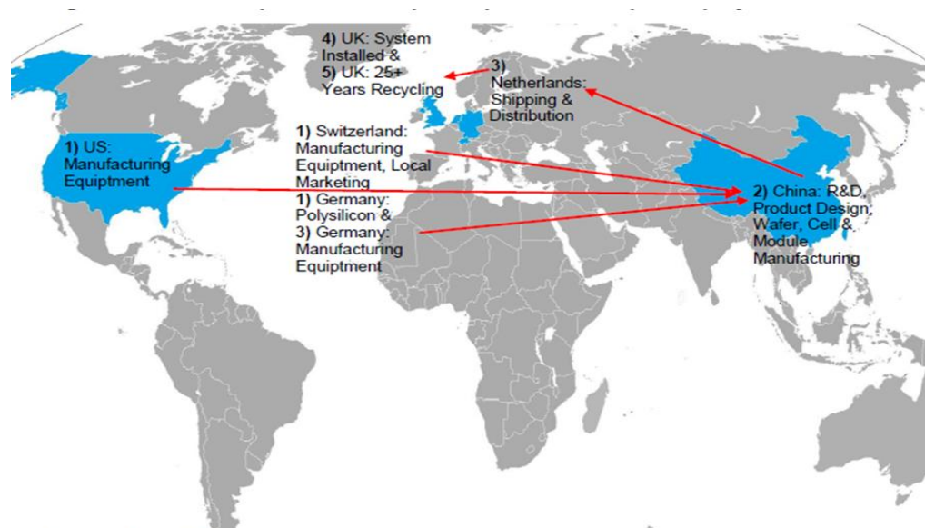
Figure 5.8 The life cycle of a solar power plant 51
